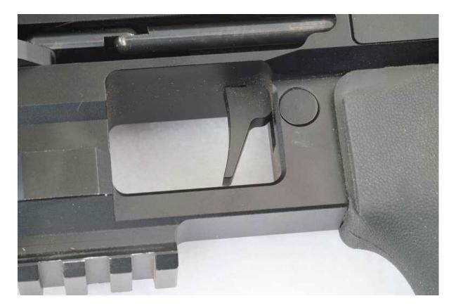
The RTI Prophet air rifle has a two-stage trigger that can be adjusted down to a pull weight of just over 10 Ounces, the company tells HAM. The pull weight of the gun tested by HAM averaged 1 Lb 12.1 Oz.
