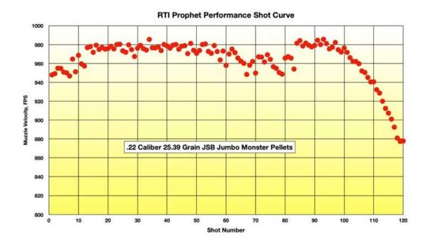
As can be seen from the chart above, the gun featured in this RTI Prophet PCP test review delivered **108 consistent shots from a full fill of it's large, 500cc carbon fiber bottle**. The HAM Team considered this to be a very good shot count for a PCP of this power level in .22 caliber.
