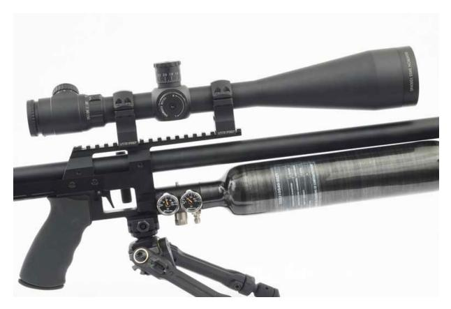
Needless to say, for such a long-range shooting combination, support is required to achieve the accuracy potential. This is where the lower Picatinny rail is most useful, as a bipod can be mounted there.
