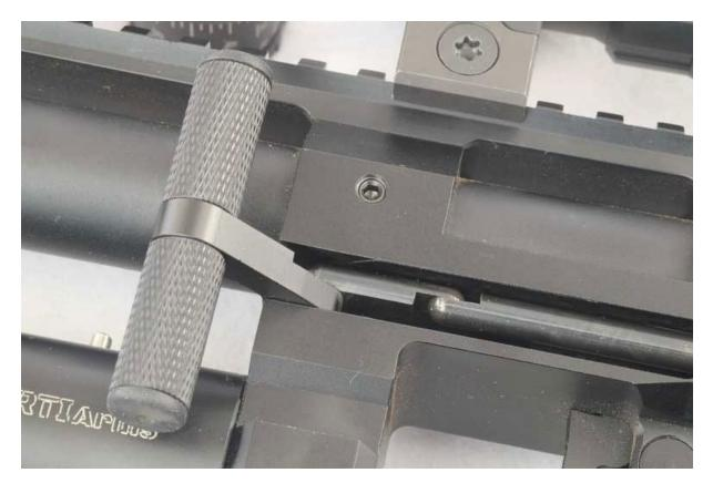
The cocking lever handle is well knurled and permits easy grasping with two fingers. After a long, easy "first stage", there's a short and quite heavy "second stage" where using two fingers is definitely beneficial.
