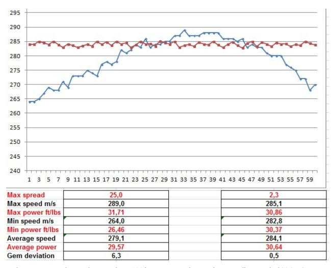
In this case we set the regulator to about 130 bar pressure, this results in a pellet speed of 285 m/s with 16 gn JSB. Of course, the regulator can be set higher or lower when you prefer a higher pellet speed.
